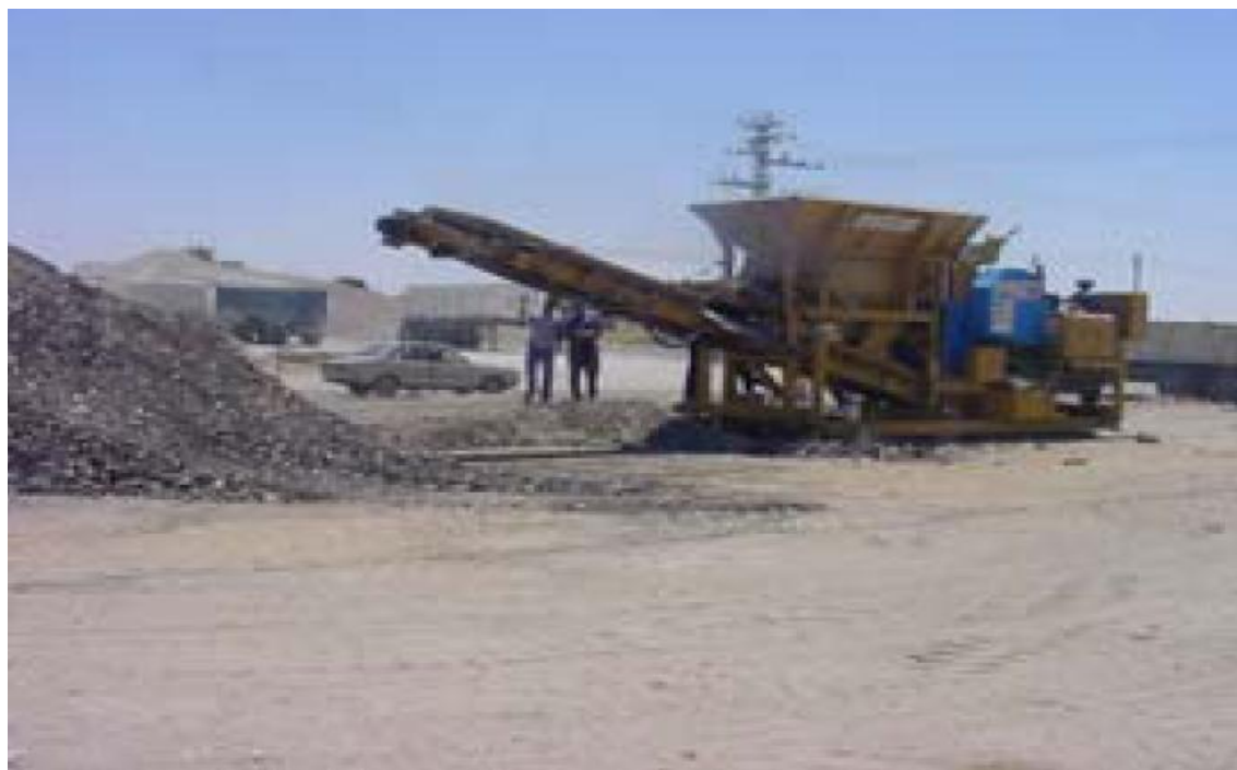
Figure 2.1 Construction and demolition waste crusher
