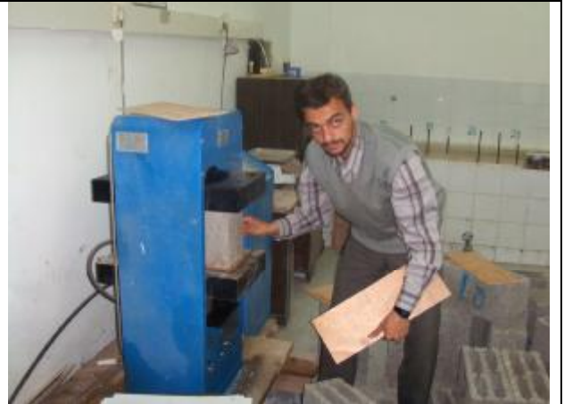
Figure B16: Block compressive strength test
