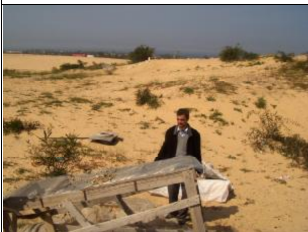
Figure B5:Sieving recycled aggregate
